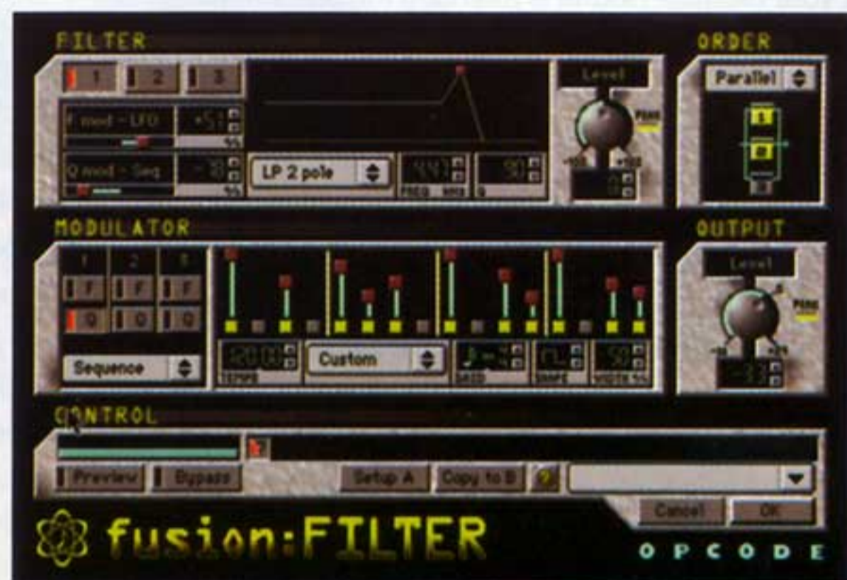
Figure 1. Fusion:Filter provides three analog-style resonant filters that can be connected in parallel or series. They can be modulated over time for rapid or slowly evolving effects that can be subtle or surprising.
