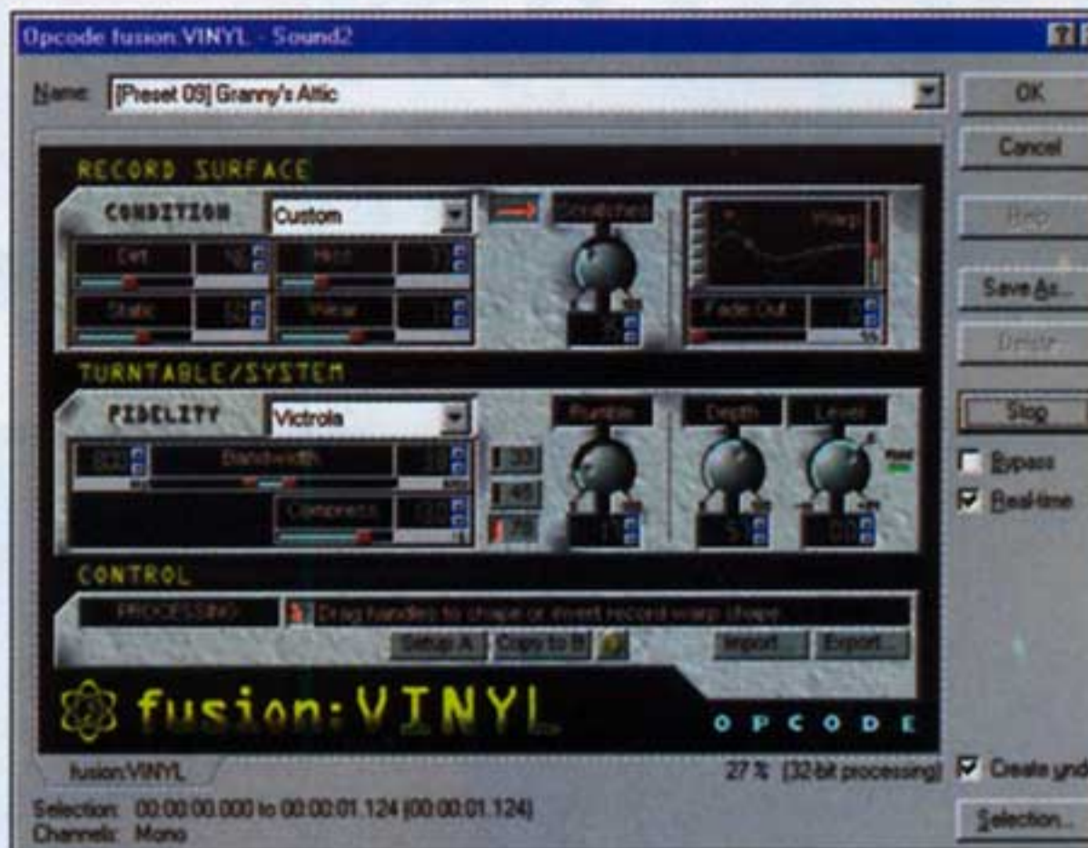
Figure 3. You can add vinyl record effects such as pops, dust, noise, and warping to any audio clip using Fusion:Vinyl. This plug-in includes useful presets that simulate the sound of an AM radio and a telephone.
