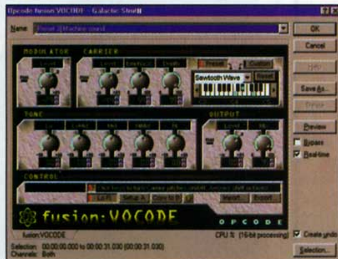
Figure 2. Fusion:Vocode allows you to impress one audio clip (such as a human voice) on another (such as a synthesized chorus) to generate vintage vocoder effects such as the classic robot voice.
