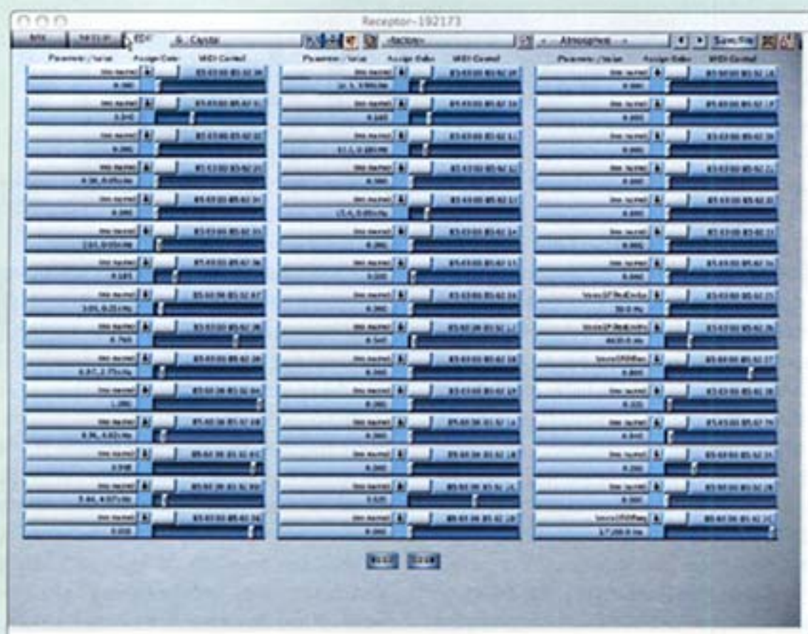
Many plug-ins can be edited in two ways: Green Oak's awesome Crystal soft synth is the example here, being edited with the barebones 'faceless' mode, which replaces the fancy graphic interface with a screen full of sliders. Some plug-ins, of course, don't have a graphic front end, leaving faceless mode as the only editing option.
