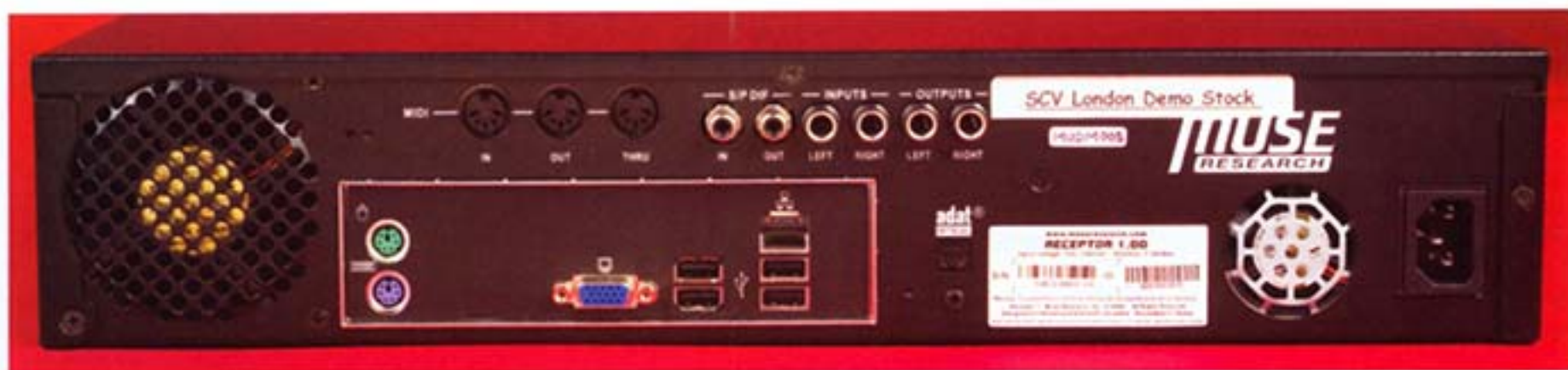
The Receptor's ADAT output currently works only in stereo mode, and if you want to expand its analogue I/O, you'll need to add a USB interface when an OS update makes this possible.
